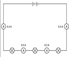
The current flowing through each lamp is less when there are more lamps, but it is still the same everywhere in this series circuit.
